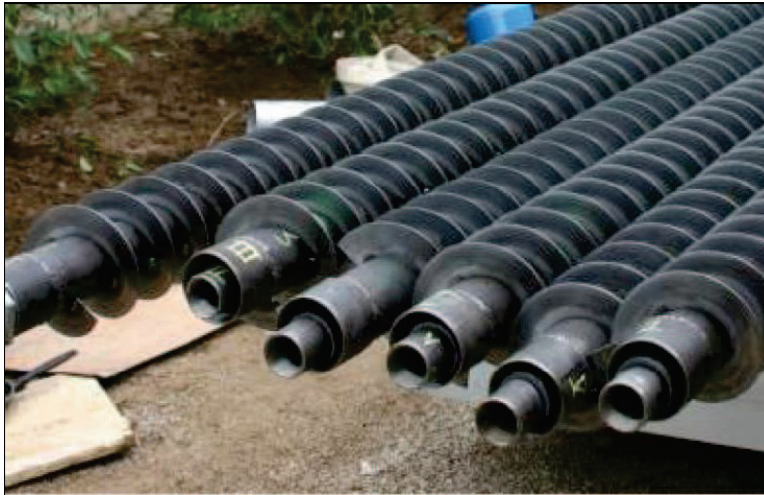
Figure 6. Inner pipe welded with steel helix, Reprinted with permission from Ref. [97], 2024, Taylor & Francis Group.
