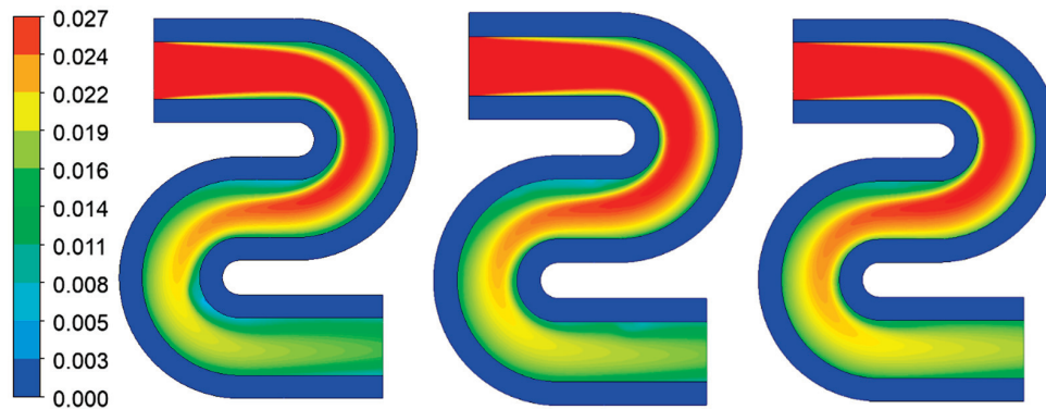
Figure 12. Mass fraction of change in wet air flow rate.
