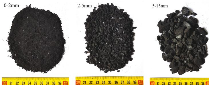
Figure 5. Screened coal particles of three different particle size classes.
