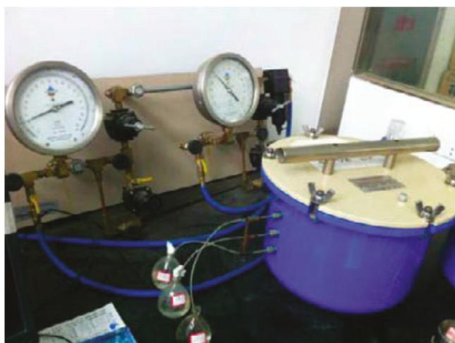
**Figure 2.** Pressure plate apparatus instrument.
