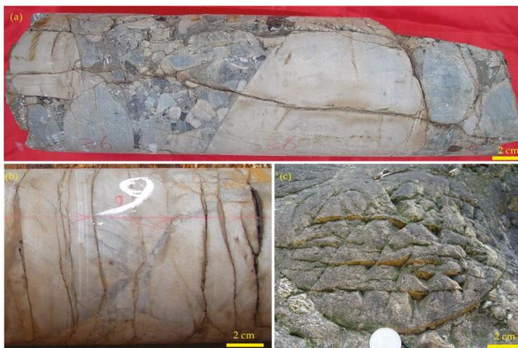
**Figure 6.** Trans-gravel fractures in cores and out crop. (a) Trans-gravel fractures with high dip angle in core, Well L102, 3185.75 m; (b) trans-gravel fractures with low dip angle in core, Well L104, 3174.65 m; (c) conjugate fractures in outcrop, see Figure 1 for outcrop location.
