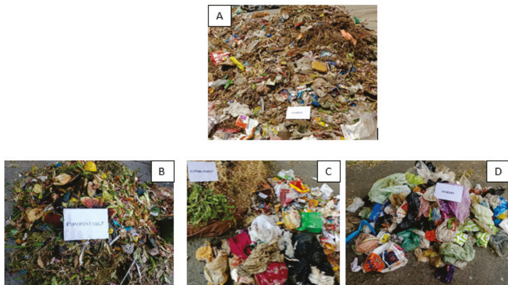
Figure 3. (A) Unsorted bulk MSW sample collected for Mehmood Booti Open dump site of Lahore; (B) compostable fraction of MSW; (C) combustible fraction of MSW; (D) components of MSW left after derivation of combustible and compostables.
