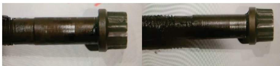
Figure 7. Patterns of the indentations on the surface of bolt screws.
