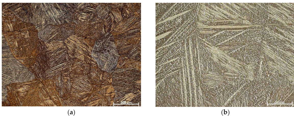
Figure 2. Microstructure of the Cu-10Al-7Ag SMA alloy in the quenched condition: (a) low-magnification polarized light OM image, (b) high-magnification bright field OM image.
