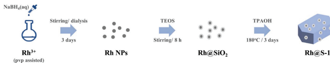
Figure 7. Schematic illustration of the steps for the preparation of the Rh@S-1 [38].
