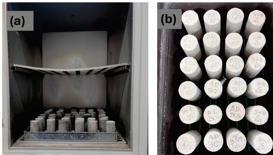
Figure 5. Oven-drying of the mortar test specimens (a); performance of the capillary water absorption test on the test specimens (b).
