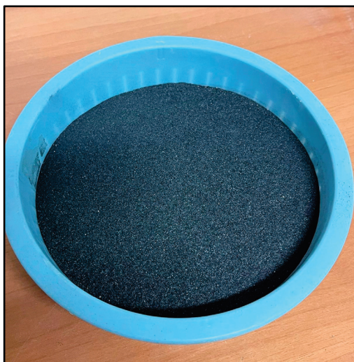
Figure 1. Mill scale: iron oxide residue generated on the steel surface during hot rolling.
