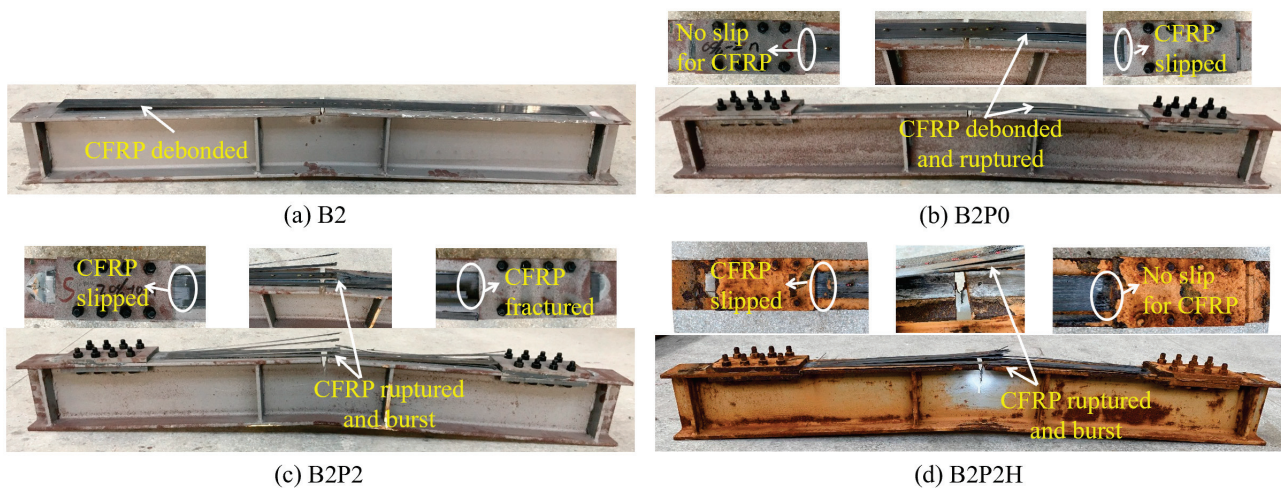
Figure 11. Failure modes of strengthened beams with Sa3 sandblasting grade.
