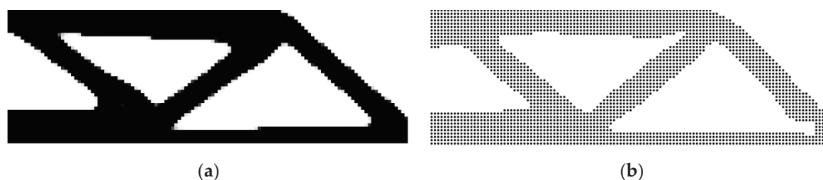
Figure 9. The optimized topologies obtained by (a) the finite element method with the elemental density variables ( c = 190.706 ) and (b) the mesh-free method with the nodal density variables ( c = 230.361 ).
