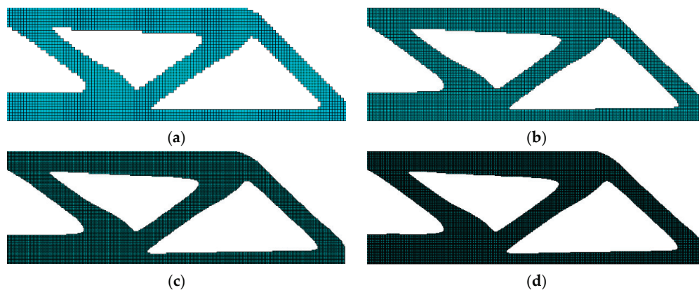
Figure 6. Optimized structures were obtained by (a) 120 \times 40 elements, c = 228.345 , (b) 240 \times 80 elements, c = 229.803 , (c) 360 \times 120 elements, c = 232.363 and (d) 480 \times 160 elements, c = 234.799 .
