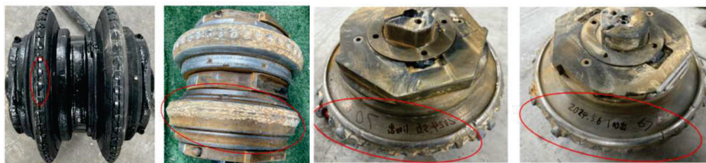
Figure 7. Hard alloy disk cutters and the alloy detached after their failure.
