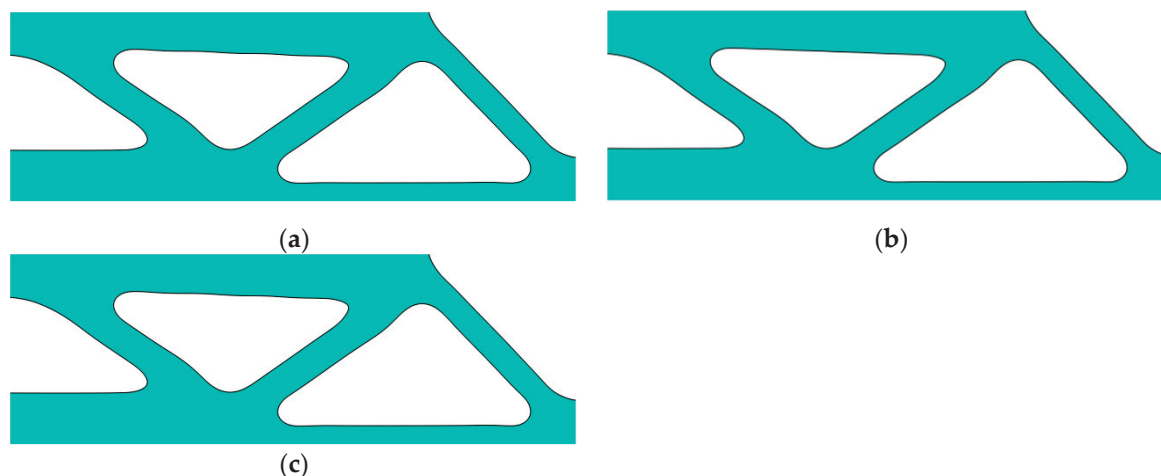
Figure 8. The optimized topologies use three different discretizations: (a) 241 \times 81 with c = 195.845 , (b) 361 \times 121 with c = 197.322 , and (c) 481 \times 161 with c = 198.598 .
