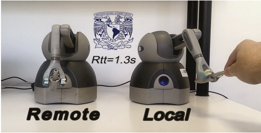
Figure 2. Teleoperation system composed of two Geomagic Touch haptic devices.
