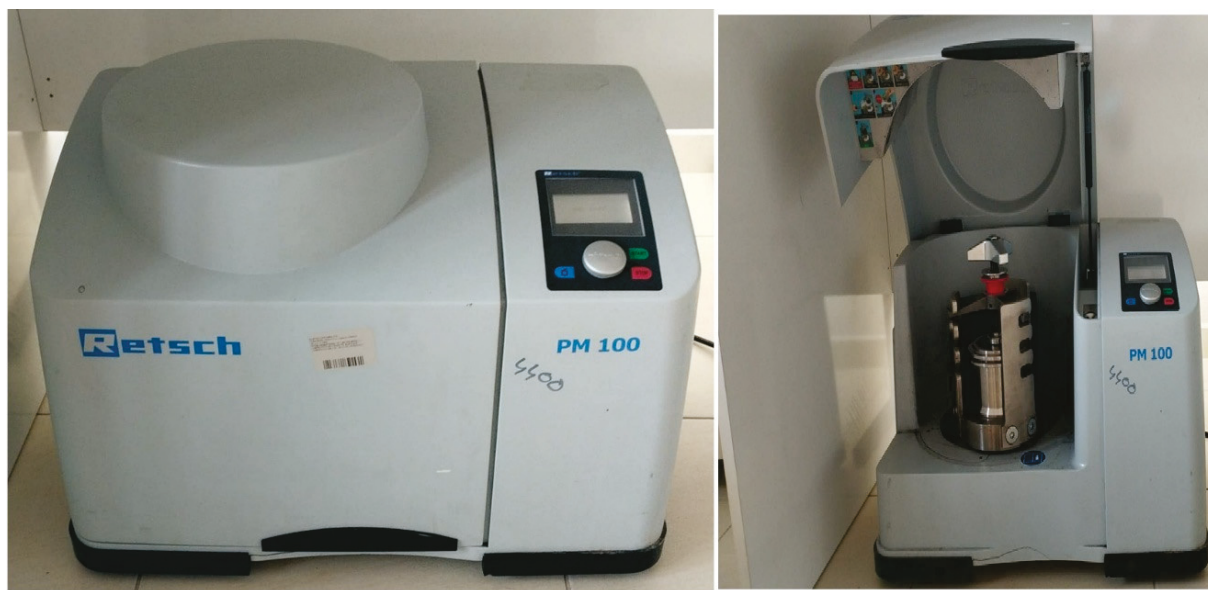
Figure 1. Retsch PM 100 planetary ball mill present in Bartın University, Turkey.
