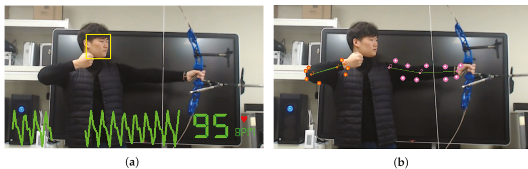
Figure 7. Examples of biometric data extraction: (a) heart rate extraction using rPPG; (b) micro-movement feature points.
