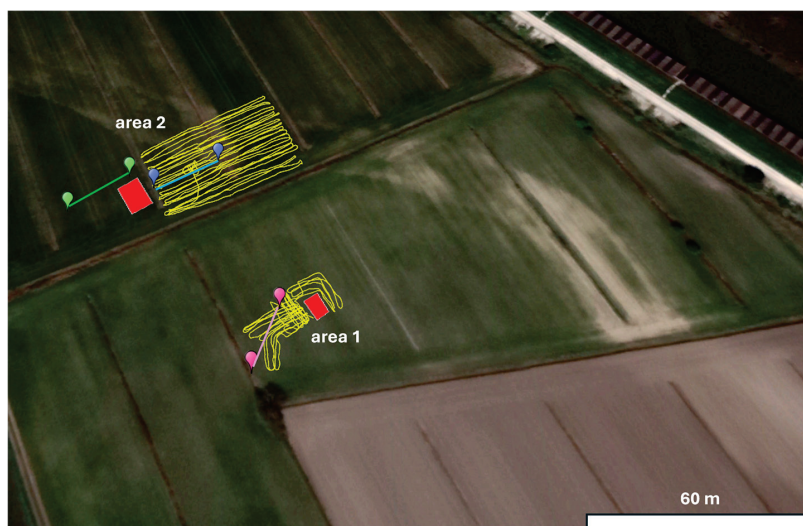
Figure 5. Locations of the FDEM measurements (yellow lines) and ERT lines (green, blue and pink) in the two excavated areas in red.
