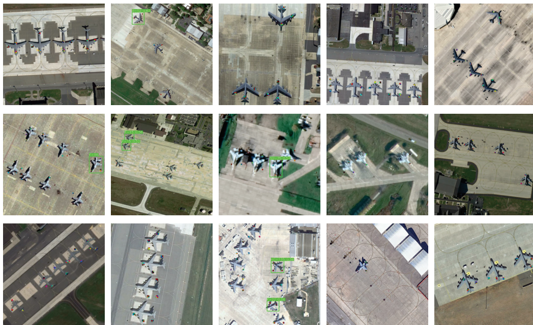
Figure 5. Visualization of adversarial attack results. Three adversarial patches are applied to each target, with each patch occupying 3% of the target's area. Green bounding boxes indicate detected objects.
