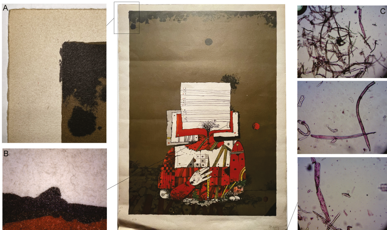
Figure 1. Selected lithograph for the study. (A) Margin detail: The paper appears to have a porous and loosely packed fiber structure. The large amount of surface dirt is visible to the naked eye. (B) Central area detail: The contrast between the surface of inked areas and the support is visible. In the red ink, less penetration of dirt is especially clear due to the smoother texture of the inked areas. The gloss effect created by overlapping of the inks, red and black in this case, is also apparent. (C) Optical microscopy fiber analysis with Lofton–Merritt staining test: results indicate that paper is made of sulfite-based bleached chemical pulp with some unbleached fibers. The fibers are in an acceptable condition. The small amount of sizing is apparent from the minimal visible residue between fibers and the ease of separation without prewashing.
