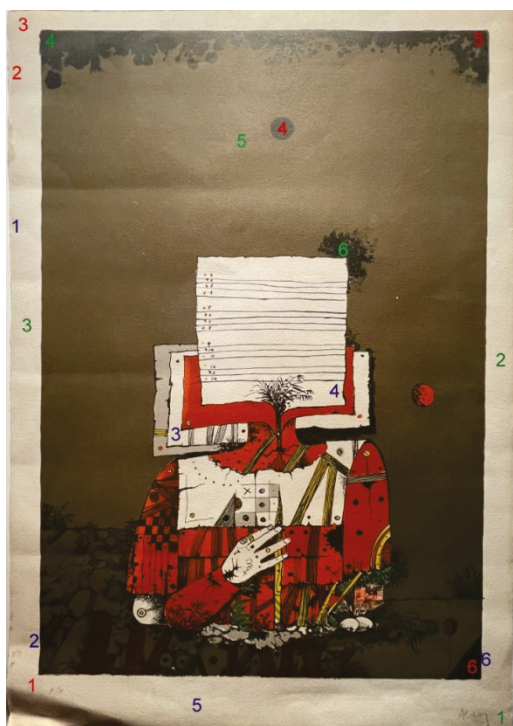
Figure 3. Location of the spots examined with each analytical technique: optical microscopy (marked in blue), scanning electron microscopy (marked in red), and spectrophotometry (marked in green).
