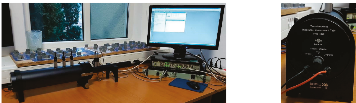
Figure 2. The Impedance Tube Kit Type 4206® (Brüel&Kjær) used for acoustical investigations.
