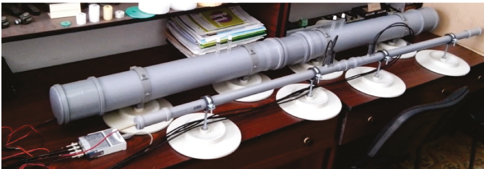
Figure 3. Transmission loss tubes used for evaluation of noise insulation ability of foams.
