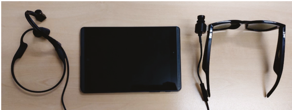
Figure 8. Two realizations of the Colorophone 2.0 system together with the processing unit in the form of a Windows tablet.
