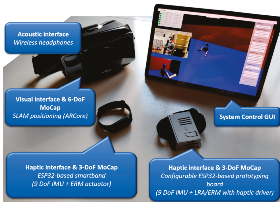
Figure 1. The VES system (the image in the tablet is a capture of the GUI and a photo of the user).
