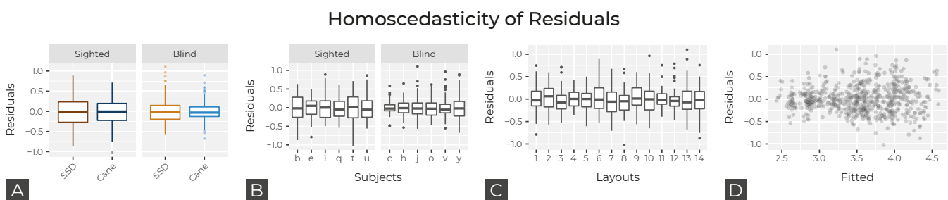
Figure A6. Graphical representations of variance between different variables to show homoscedasticity/homogeneity of variance: (A) group and aid, (B) subjects and (C) layouts. Furthermore the residuals vs. fitted scatterplot in (D) allows to check for non-linearity, unequal error variances and outliers. Even though the variances of the error terms seem to be slightly left-slanted, the data can be seen as reasonably homoscedastic and homogeneous.
