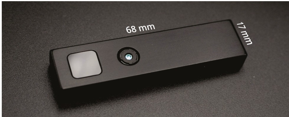
Figure A1. The chosen ToF camera development kit Pico Flexx from pmdtechnologies.
