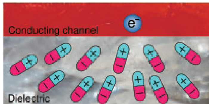
Figure 8. Sketch of the effects induced by the charge carrier in the conducting channel on the gate close to the interface. The electron in the organic semiconductor induces a polarization within the dielectric that, in turn, affects the electron dynamics.
