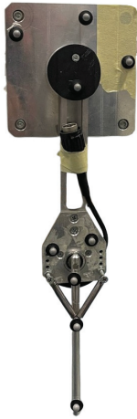
Figure 2. Experimental setup: the 2-DOFs underactuated manipulator.
