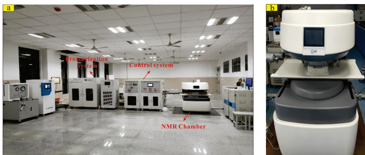
Figure 1. Variable-temperature high-pressure nuclear magnetic resonance (NMR) analysis system: (a) NMR system; (b) NMR chamber.
