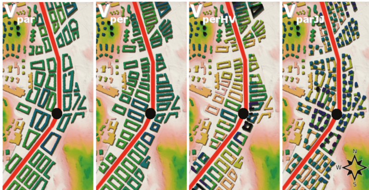
Figure 1. The city-block-design alternatives. From left to right: V_{par} (the longer sides of buildings parallel to the boulevard), V_{per} (the longer sides perpendicular to the boulevard), V_{perHV} (similar to V_{per} but the building height varies) and V_{parJJ} (similar to V_{par} but with Jing-Jang building structure variation). The boulevard is marked in red and the major junction with a black dot.
