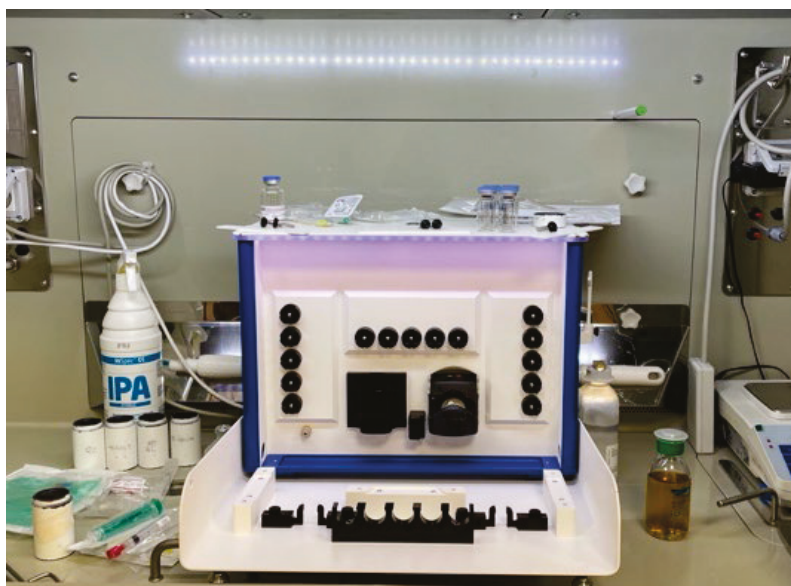
Figure 9. Example of a synthesis module for the preparation of ^{68}\text{Ga} radiopharmaceuticals, installed within a shielded hot cell in a hospital radiopharmacy. The module is equipped with pre-defined positions for reagents, cassettes, and waste containers, enabling standardised and operator-independent execution of radiolabelling procedures under aseptic and radiologically safe conditions.
