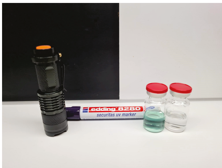
Figure 3. UV lamp and UV marker with two vials from the final GMP QTSs filled with either WFI + fluorescent dye IRDye 800CW (left vial, colored solution) or WFI (right vial, clear solution).
