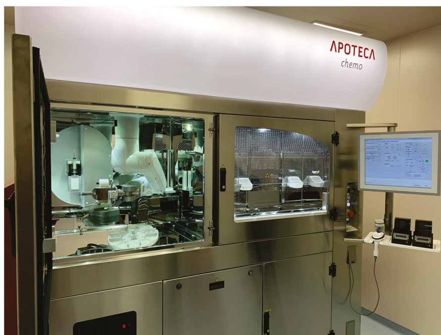
Figure 4. Reconstitution robot at the Department of Clinical Pharmacology and Pharmacy, Amsterdam University Medical Center, location Vrije Universiteit (photograph: MC).
