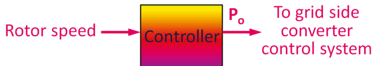
Figure 8. Power Signal Feedback Control Block Diagram.
