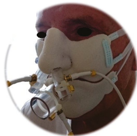
Figure 1. Placement of the printed mask with sensors on the patient's face.
