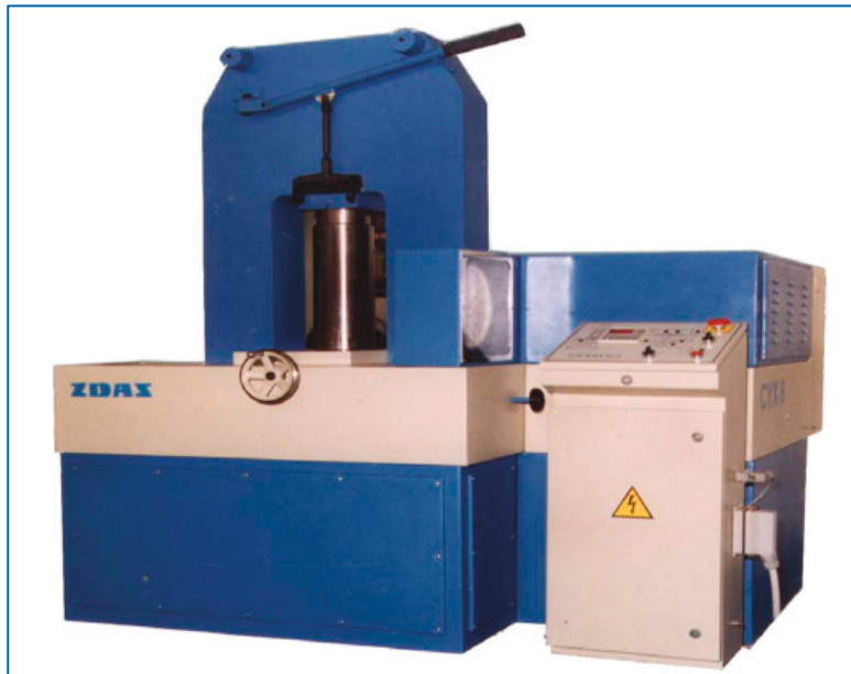
Figure 3. The high-pressure isostatic press CYX 6/103 (Žďas join-stock company, Žďár nad Sázavou, Czech Republic).
