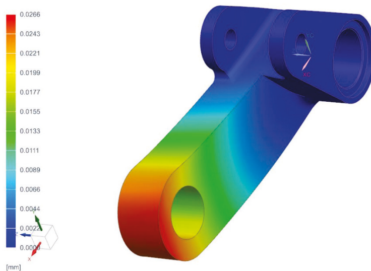
Figure 7. Color distribution of the displacement on the model.
