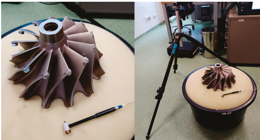
Figure 2. Experimental modal analysis of a turbine wheel using hand-guided modal hammer excitation.
