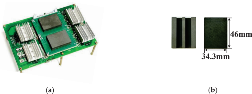
Figure 14. The experimental prototype of the DCI CF-DAB converter. (a) Top view of complete converter. (b) Optimized core shape.
