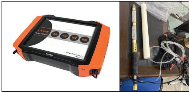
Figure 19. YL-LCT single-transmitter dual-receiver sonic probe.
