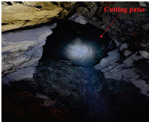
Figure 23. Blasting effect of the 2# stope cutting patio.
