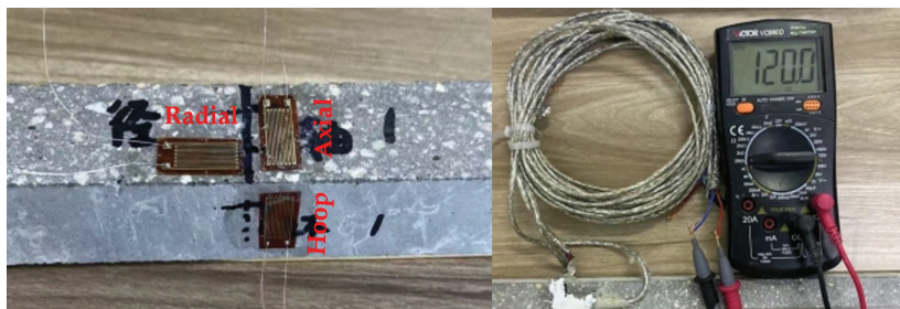
Figure 17. Strain bar, strain gauge and resistance testing.
