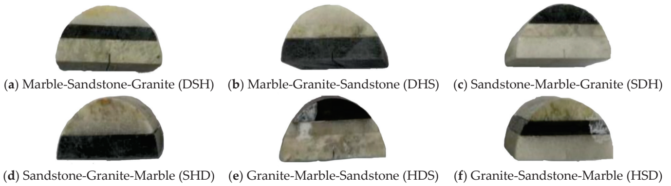
Figure 2. Physical drawing of three-layer composite rock specimen.
