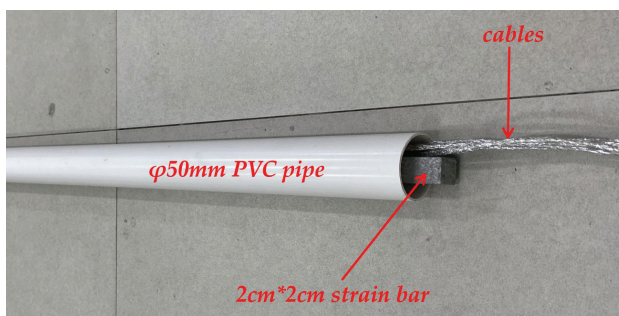
Figure 18. Schematic diagram of strain bar installation into borehole.
