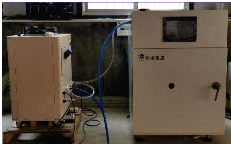
Figure 3. Multimode industrial microwave oven equipment.
