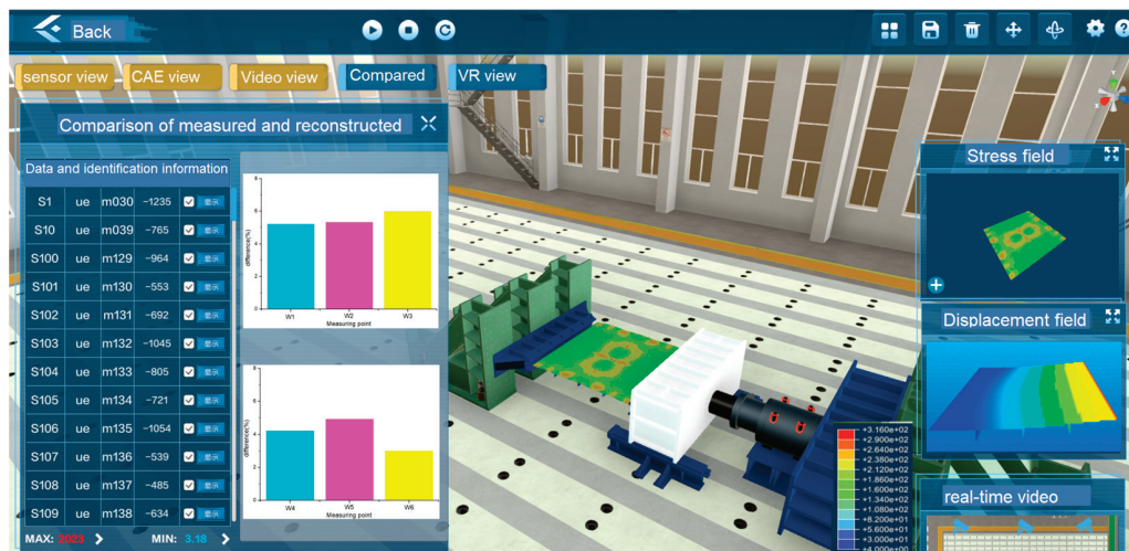
Figure 14. Real-time digital twin platform for ship structure mechanic testing.
