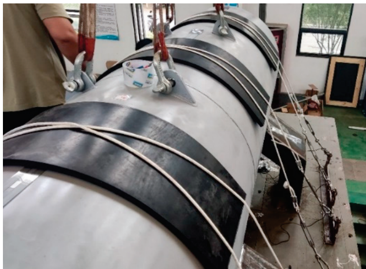
Figure 5. Tie rope ballast arrangement.
