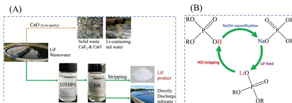
Figure 6. (A) Schematic diagram of recovery [36]; (B) mechanism of D2EHPA extract of \text{Li}^+ [36]. Reproduced with permission from Elsevier , 2023.
