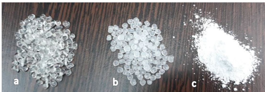
Figure 1. Raw materials used to obtain composite materials: (a) TPU beads; (b) PP beads; (c) BaTiO 3 powder.
