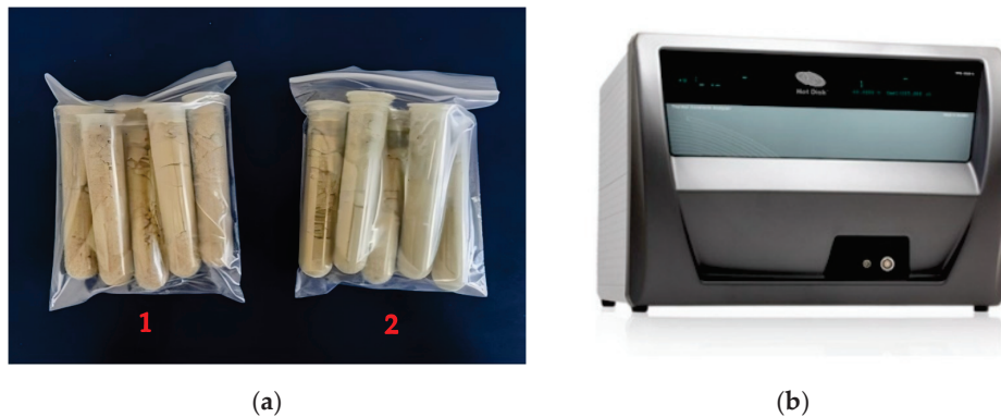
Figure 4. Thermal conductivity test sample and Hot Disk thermal constant analyzer: (a) thermal conductivity test samples; (b) Hot Disk thermal constant analyzer.
