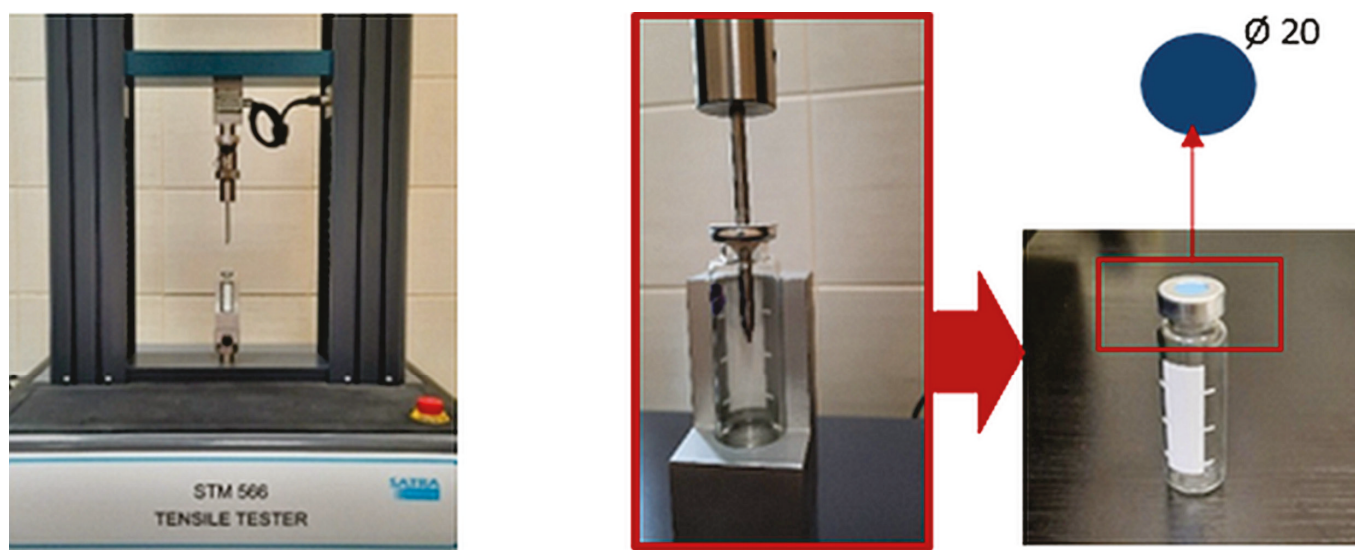
Figure 9. Measurement stand for determining chemical degradation according to EN ISO 374-4:2019 (Satra Technology, Kettering, United Kingdom).
