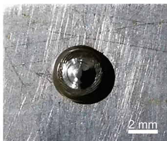
Figure 4. Appearance of 1.5 mm diameter steel ball welded onto 0.6 mm thick sheet.
