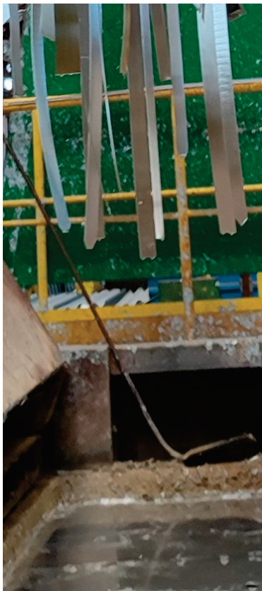
Figure 4. Samples after hot-dip galvanizing (photo by author).
