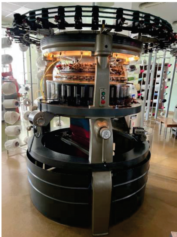
Figure 9. The Mayer & Co knitting machine used in the work to create a transmission line.
