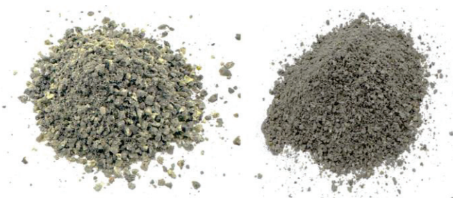
Figure 2. Bottom ash before and after the crushing process.
