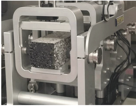
Figure 6. Testing apparatus of 4PB test.
