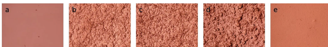
Figure 1. Surface morphology of PBAT/TPS films; glycerol/citric acid/stearic acid and ATBC serve as the plasticizers of TPS, respectively, PBAT (a), PBAT/TPS-10%ATBC (b), PBAT/TPS-20%ATBC (c), PBAT/TPS-20% glycerol (d), PBAT/TPS-30% glycerol (e).
