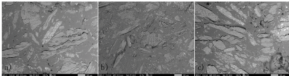
Figure 3. SEM images of the (a) reference sample (0%TW), (b) 40%TW-225 °C, and (c) 40%TW-300 °C at 100 \mu\text{m} magnification.
