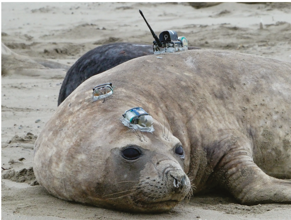
Figure 2. A female SES with three biologging devices glued: a head-mounted DTAG-4, a back-mounted CTD-SRD, and a neck-mounted SPOT. The main characteristics of the devices are listed in Table 2.
