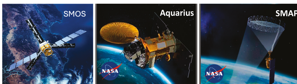
Figure 1. Artistic view of the three L-band satellite radiometers measuring sea surface salinity. From left to right: SMOS, Aquarius, and SMAP.
