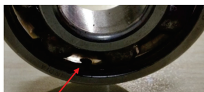
Outer race defect
