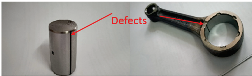
Figure 9. Crank pin and connecting rod defect.
