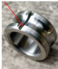
Figure 7. Inner race defect.
