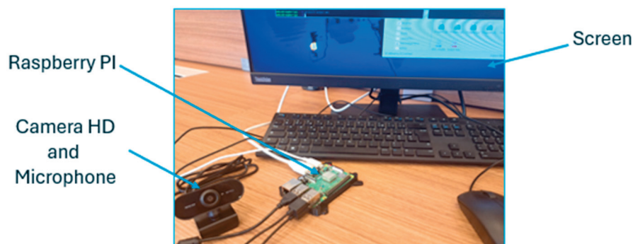
Figure 7. The hardware configuration of our system.
