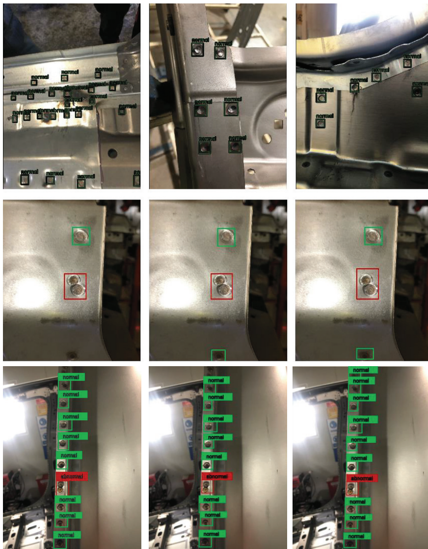
Figure 7. Some results of WSDDM and comparison between small welding spot detection models. We use green to represent the detected weld spots are normal, and red to represent the detected weld spots have defects or abnormalities.
