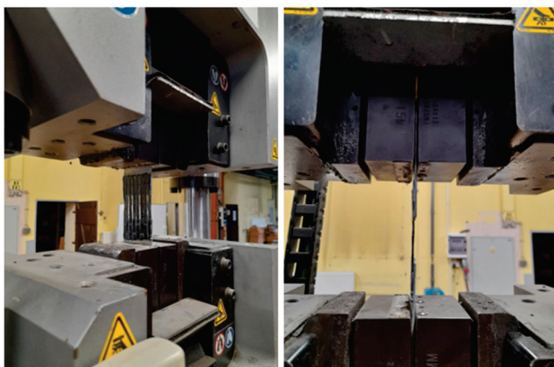
Figure 3. Specimen in the grips of a testing machine.
