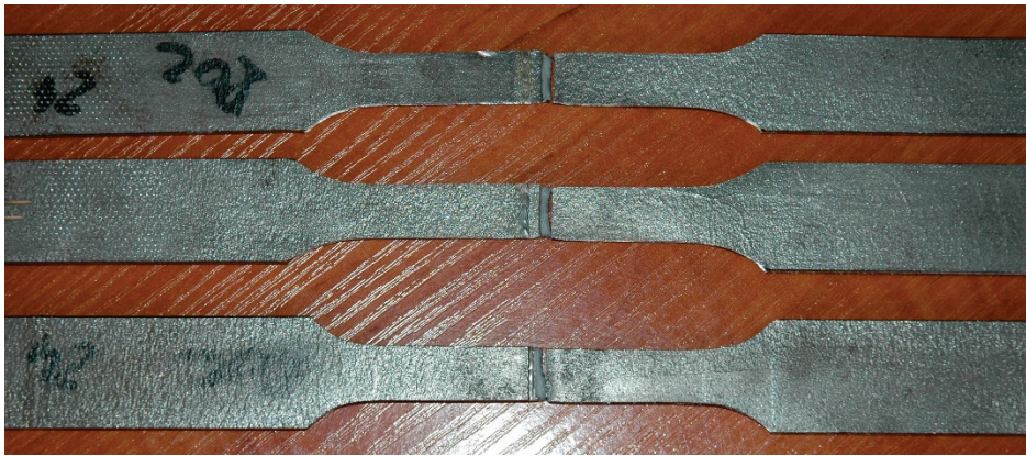
Figure 15. A view of broken samples after the static tensile tests of butt joint of ArmoX 500T steel produced via autogenous laser welding (Table 4) at lowest energy input of 70 J/mm.
