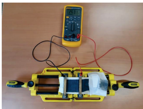
Figure 5. Two-point method resistance measurements set-up.
