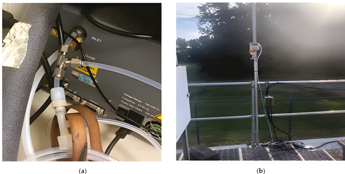
Figure 4. Photographic documentation of the MIRA Strato intercomparison with the Picarro G2301 conducted at HUBC in September 2023. (a) Inlet tubing configuration connecting the MIRA Strato and Picarro G2301 analyzers to a shared ambient intake line. (b) Tubing outlet positioned on the rooftop of the HUBC MDE monitoring site, demonstrating the shared ambient air intake configuration for comparative analysis.
