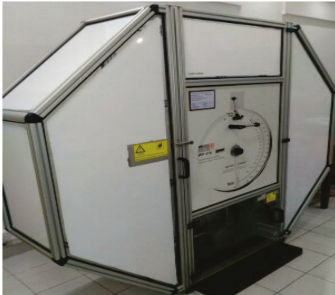
Figure 4. Impact testing machine used in the research (GUNT WP410).
