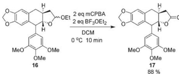
**Scheme 10.** Lewis acid and mCPBA mediated oxidation of an ethoxytetrahydrofuran to the corresponding lactone.
