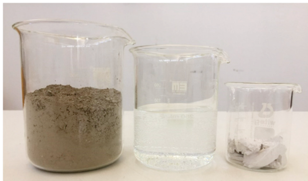
Figure 3. Raw materials: ordinary Portland cement ( left ), water ( middle ), and waste marble slurry ( right ).
