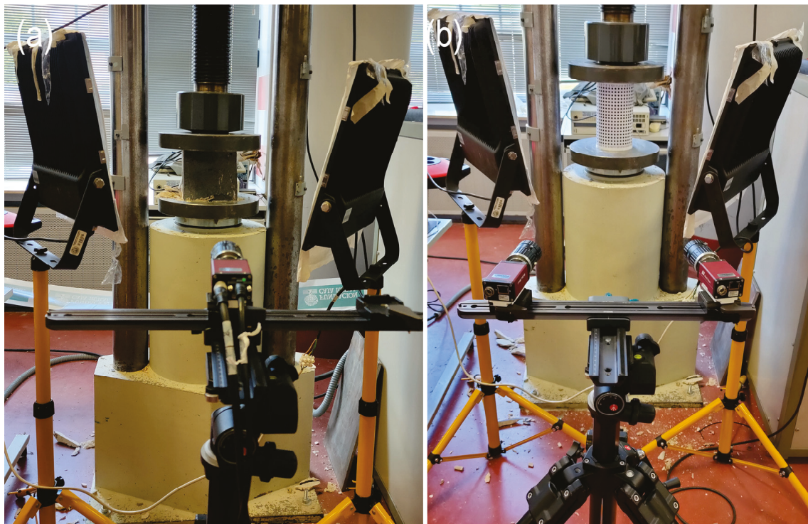
Figure 4. Digital image correlation prototype: (a) 2D-DIC; and (b) 3D-DIC.
