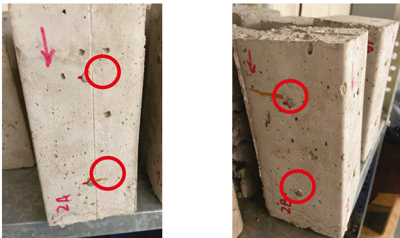
Figure 4. Concrete samples for shrinkage measurements. Reference points marked with red circles.
