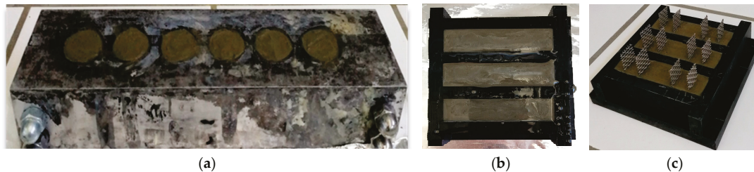
Figure 4. Casting of cement paste specimens in (a) cylindrical and (b) prismatic molds and (c) with embedded grids for resistivity measurements.
