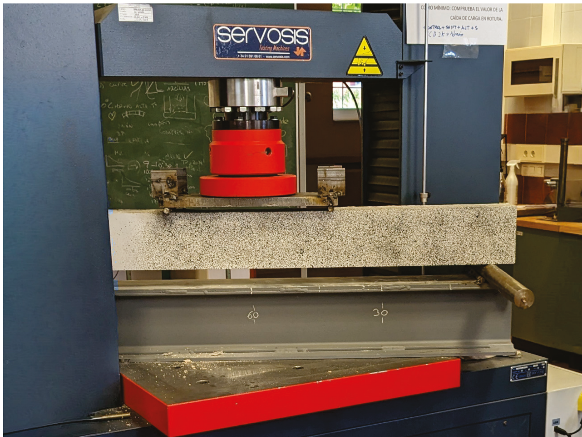
Figure 6. Platform and set up for four-point bending test of beam prototypes.
