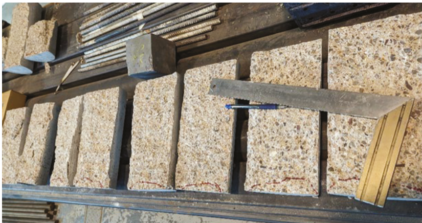
Figure 5. Concrete samples after water penetration depth measurements.
