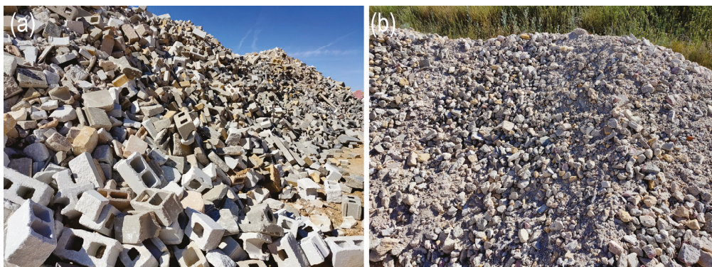
Figure 1. Rejection of the manufacture of prefabricated products with siliceous aggregates: (a) prefabricated elements; and (b) crushed aggregates.
