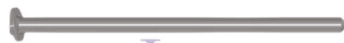
Figure 1. This figure shows the SI screw with a washer used to simulate the USI, BSI, and TSI.
