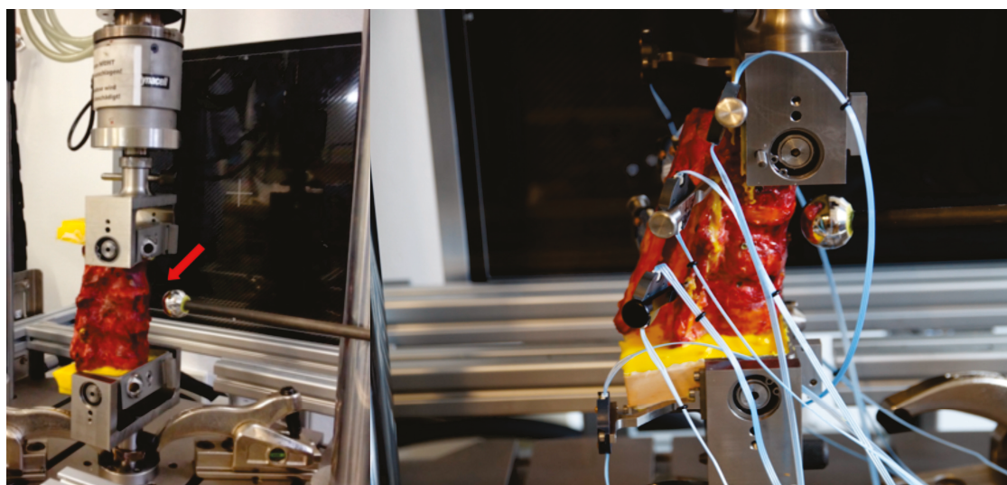
Figure 2. Hydraulic material testing machine used to create standardized incomplete burst fractures and obtain radiographs. At the left , the mounted motion capture marker (rigid bodies) and radio-graphic reference (arrow) are shown. At the right is a magnified lateral view of a mounted sample.
