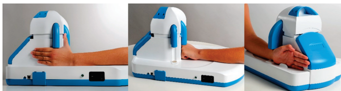
Figure 1. BAUSport™ SonicBone device protocol (1st, 2nd and 3rd hand measurements positions) (source: https://sonicbonemedical.com/product/ , accessed on 30 January 2025).
