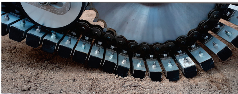
Figure 10. Detailed photo of the track belt.
