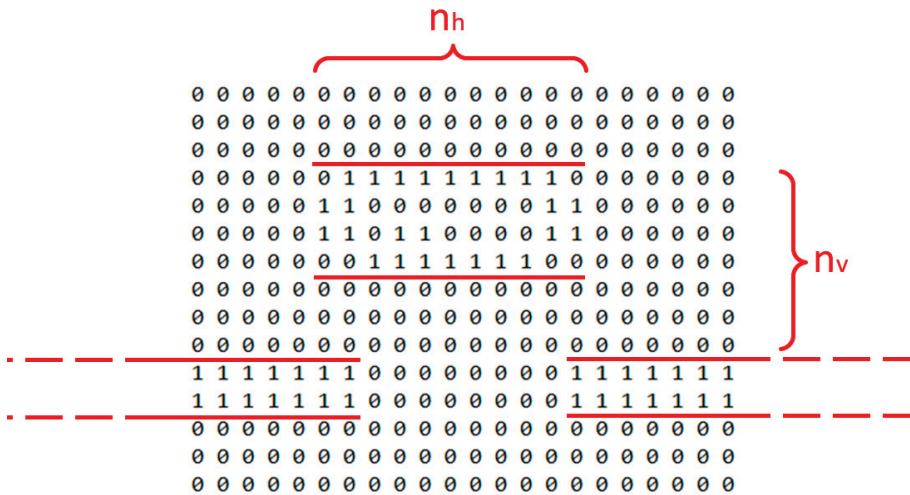
Figure 15. Obstacle width and height of pixel selection from the processed image (red lines represent laser linear projection width).
