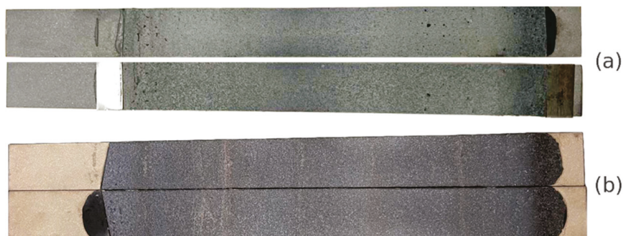
Figure 17. Failure mode of the DCB specimens for (a) Adhesive A and (b) Adhesive B, showing cohesive failure for both adhesives.
