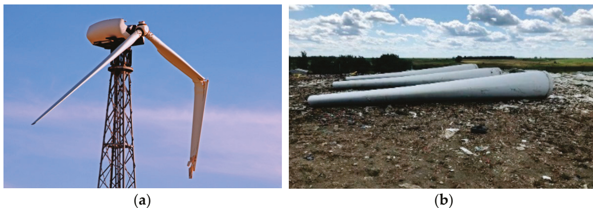
Figure 1. Illustration of two critical problems of wind energy: (a) Wind turbine with broken blades, and (b) wind blades accumulated in landfill. Photos from Bigstock © collection.
