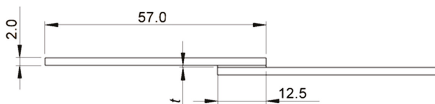
Figure 7. Dissimilar SLJ geometry. The width of each adherend is 12.5 mm, and t represents the thickness of the adhesive layer.
