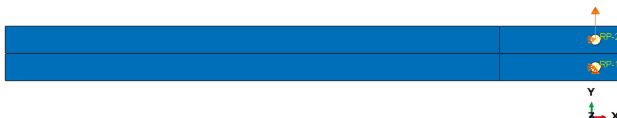
Figure 11. Boundary conditions for the DCB model.
