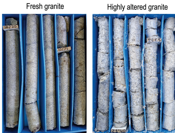
Figure 2. Boreholes of fresh and highly altered granites.
