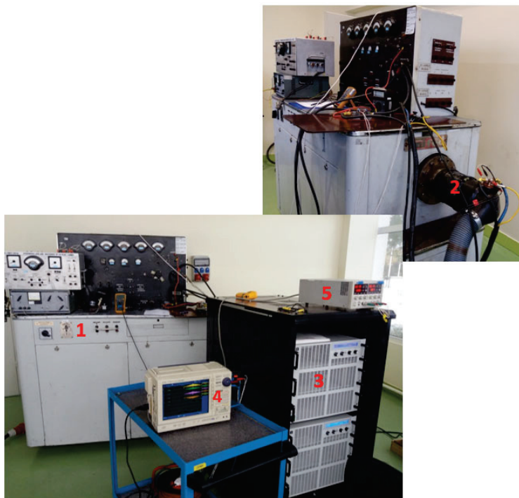
Figure 9. View of the VR-600 test stand for testing GS-12T 3s DC generators: 1—VR-600 drive stand, 2—GS-12T 3s generator under test, 3—EL 9080—600 HP thyristor load, 4—oscilloscope, 5—DC power supply.
