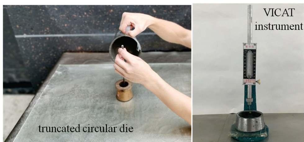
Figure 3. Setup of truncated circular die and VICAT instrument.
